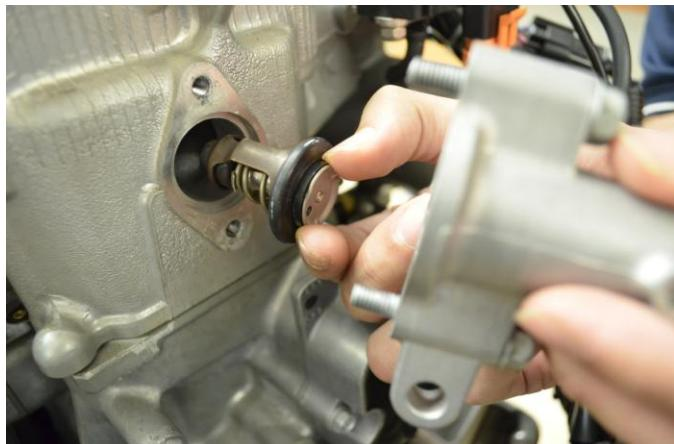
Clean thermostat opening of any corrosion to ensure proper sealing of o-rings on restrictor.
